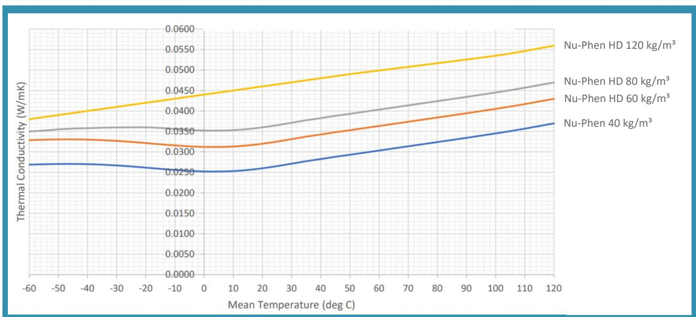
**Nu-Phen HD** is a closed cell, thermally efficient rigid foam, based on phenolic resins and containing no CFC's.
